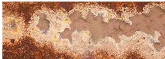
It is the chemical and physical interaction between a metal and a water-based medium, which causes changes in the properties of the metal and which often leads to a loss in the functionality of the metal itself, of the medium or of the system consisting of these two elements.
