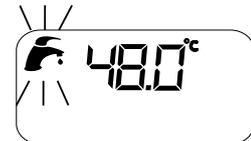
7. To adjust the heating water temperature press heating water temperature buttons (**6** in fig. 1); then set as required. While the heating water temperature is being regulated, the LCD displays the temperature setting and the CH symbol flashes.
